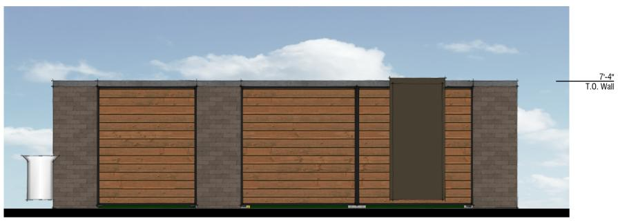
Trash Enclosure - West Elevation 1/4" = 1'-0"
