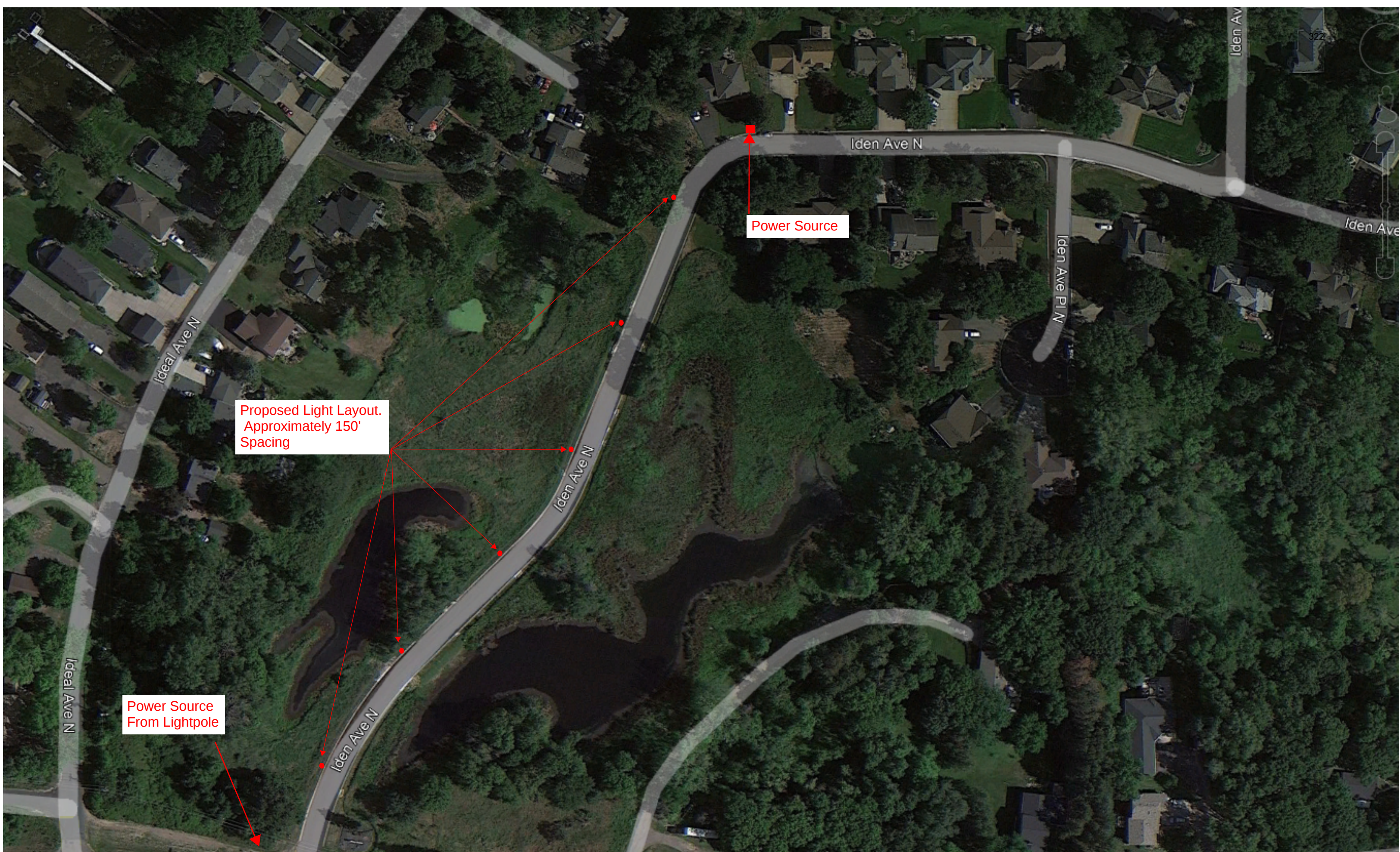
PIONEER POINT PROPOSED STREET LIGHT LAYOUT
