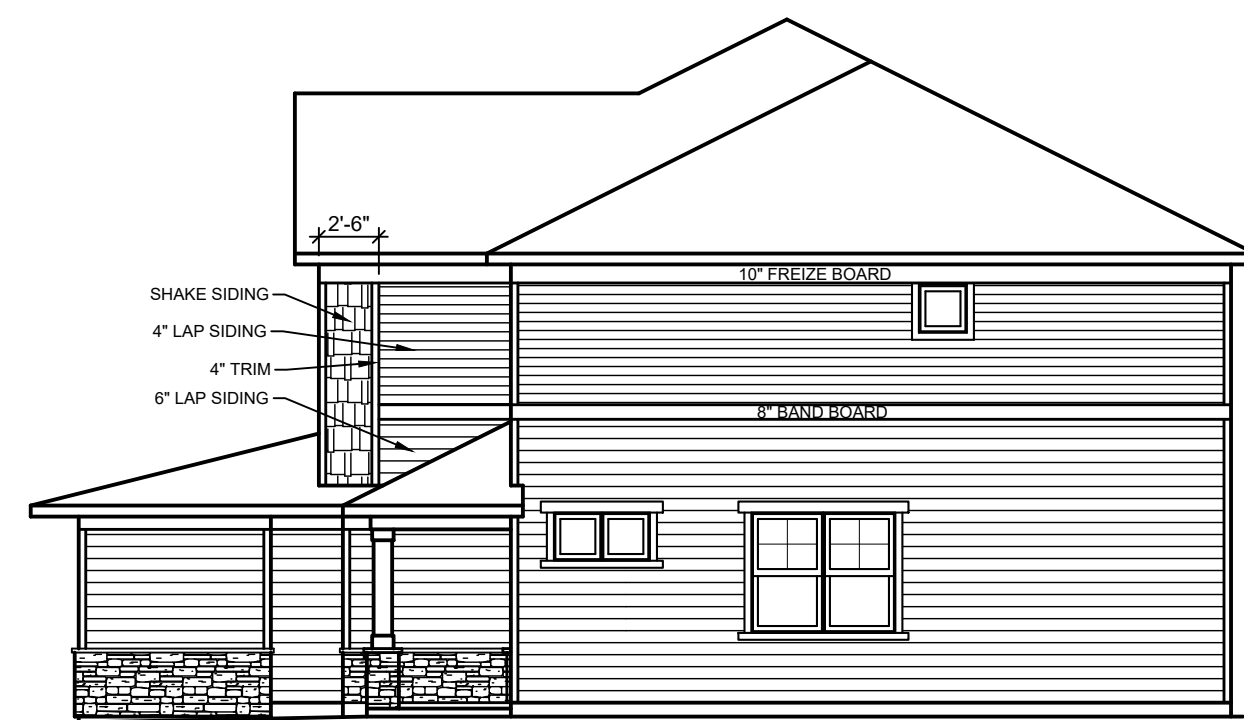
2 SIDE ELEVATION - SIDING END - GARAGE LEFT SCALE: 1/8" = 1'-0"
