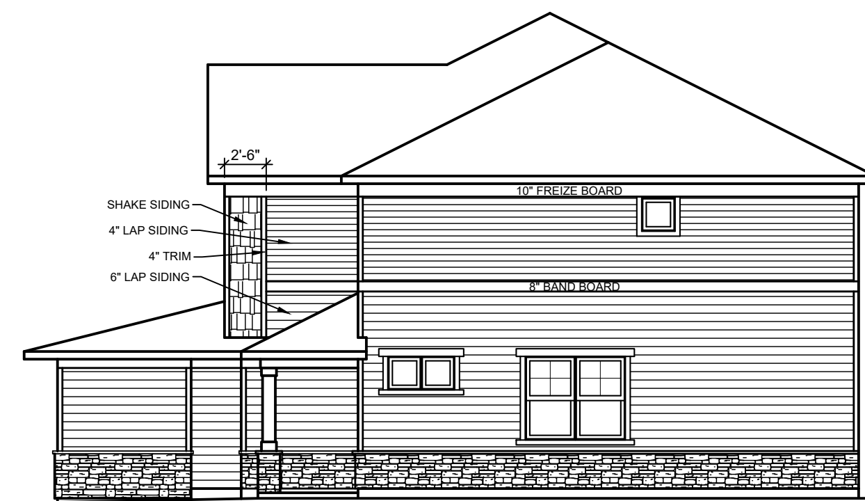
3 SIDE ELEVATION - STONE END - GARAGE RIGHT SCALE: 1/8" = 1'-0"
